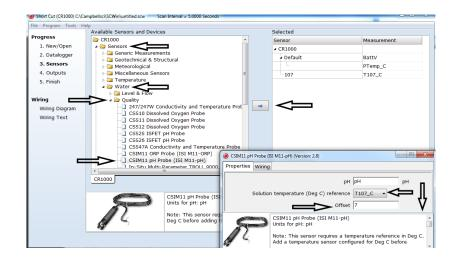
7. After selecting the sensors, click at the left of the screen on **Wiring Diagram** to see how the sensor is to be wired to the datalogger. The wiring diagram can be printed out now or after more sensors are added.
