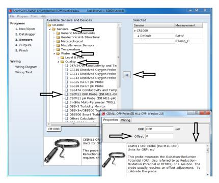
6. After selecting the sensors, click at the left of the screen on **Wiring Diagram** to see how the sensor is to be wired to the datalogger. The wiring diagram can be printed out now or after more sensors are added.
