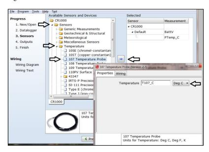
Ouality folder. Select CSIM11 pH Probe. Click to move the selection to the Selected device window. Click on the Solution temperature (Deg C) reference box and select T107\_C. The probe usually requires an offset adjustment. The white panel at the bottom of the Properties window provides a procedure for determining the value that should be entered in the Offset box.
